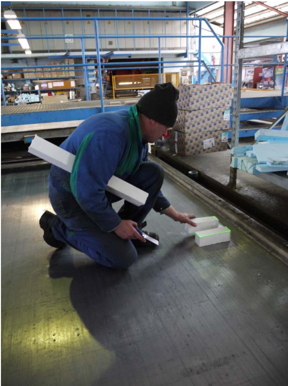
A clearly visible laser line marks the target position to the exact millimetre and facilitates precise working
