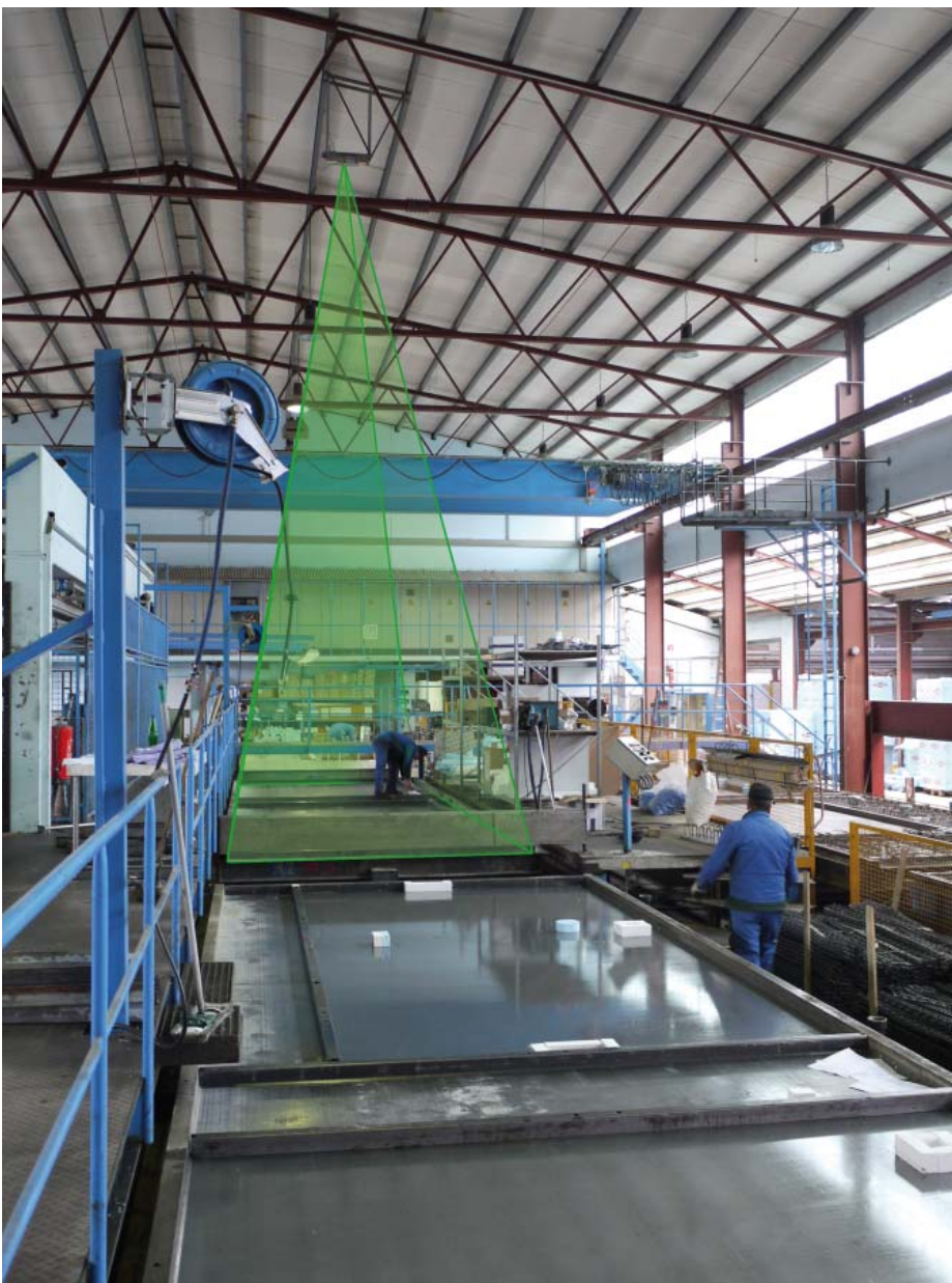
The projector is mounted at a height of around nine metres above the crane track at the first placement station
