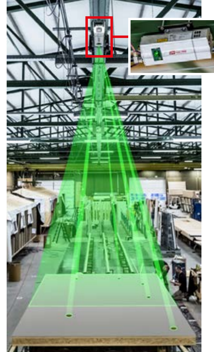
The CAD-PRO laser projection system is mounted above the work surfaces and enables precision laser projection onto flat roof elements from a distance of several meters.
