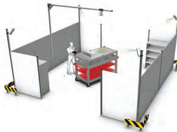
Fig. 2: Manufacturing cell with projection lasers and camera system
