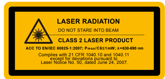
Fig. 8: Sample laser warning sign per EN 60825-1. The laser class must also be clearly marked on the laser.
