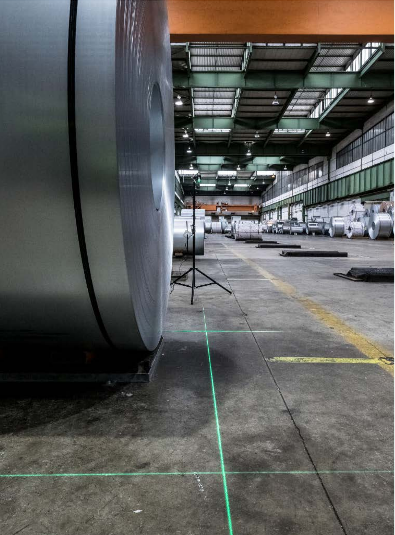
Line lasers generate colored marking lines that are always visible, even in heavily stressed areas.
