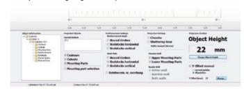
With checkboxes you can select which elements of the whole object should be projected. If you move the mouse pointer over single items in the tree structure, you will get a pop-up window with detailed Unitechnik data of this item.
