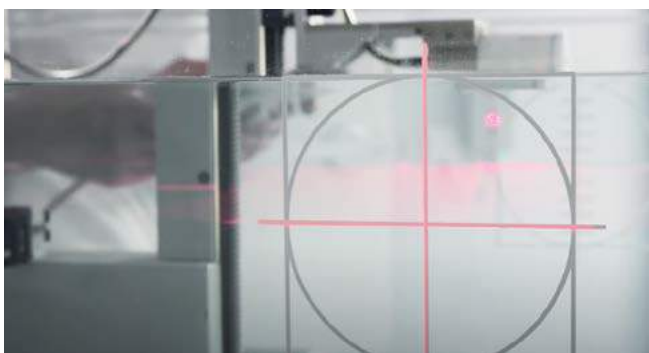
Laser-based alignment of the water phantom
